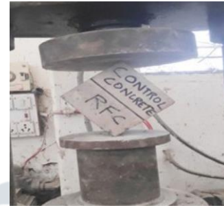
Fig. 2. Splitting Tensile Strength Test [35].
