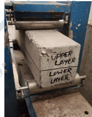
Fig. 10. Flexural Strength Test [35].
